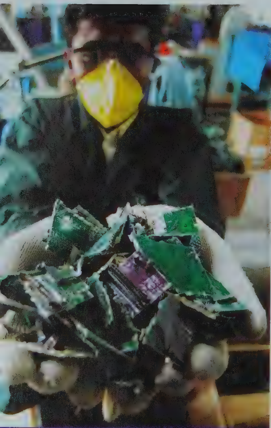
A worker at an e-waste recycling company in Bangalore, India, shows shredded pieces of printed circuit boards of obsolete electronic gadgets undergoing the recycling process. E-waste is a growing environmental and public health concern.
